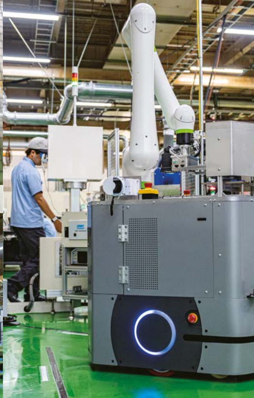
AMR (autonomous mobile robot) is in operation.
